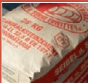
Brown sack paper is used primarily for powdered products such as cement, where the paper needs to be strong and highly porous.
